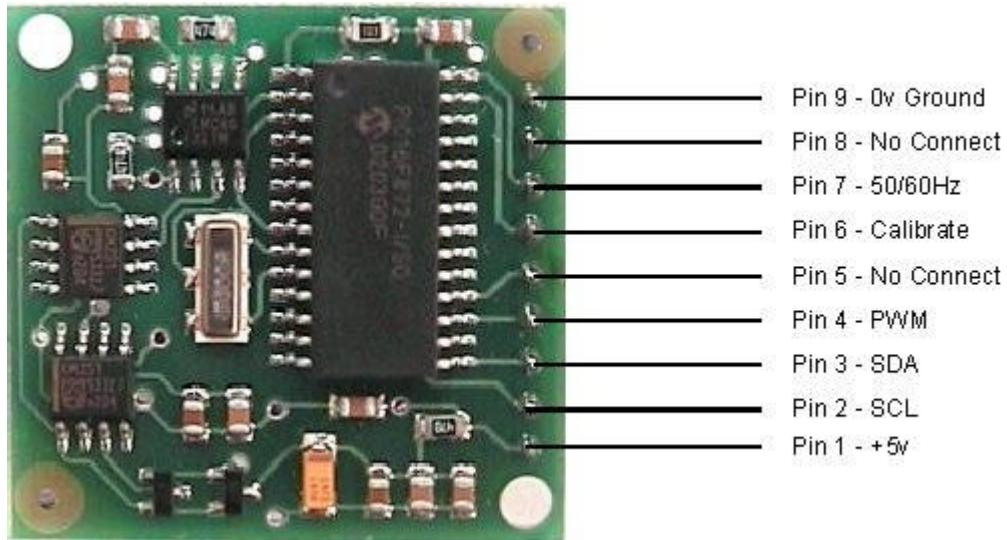
The compass module requires a 5v power supply at a nominal 15mA. There are two ways of getting the bearing from the module. A PWM signal is available on pin 4, or an I2C interface is provided on pins 2,3.
