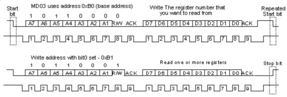
I2C communication protocol with the MD03 module is the same as popular eeprom's such as the 24C04. To read one or more of the MD03 registers, first send a start bit, the module address (0XB0 is the base address) with the read/write bit low, then the register number you wish to read. This is followed by a repeated start and the module address again with the read/write bit high (0XB1). You now read one more registers. The MD03 has 8 registers numbered 0 to 7 as follows;
