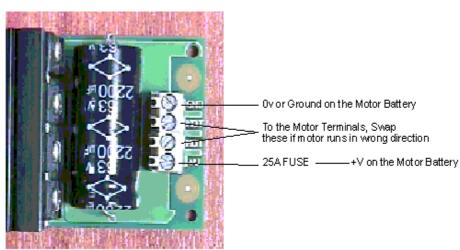
Be sure to use cable rated for at least 25/30A for the Battery, Fuse and Motor leads.
