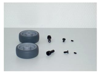
First of all, the small setscrew should be screwed into the side of the wheel bush. Next, the wheel bushes should be pushed as far as possible into the wheels, so that the countersunk screw M4 can be inserted from the other side. This is then tightened with the appropriate hexagonal wrench.
