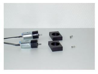
The motors are located in the large recess of the motor mounts and tightened using the small screws M2x6. Take care with plastic threads – do not overtighten the screws!
