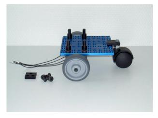
First, one of the three screws M6x10 is screwed firmly into the single threaded hole located in the plate. Then, in the same way as for the support wheel, the plate is placed on top of the base plate and screwed on from below:
