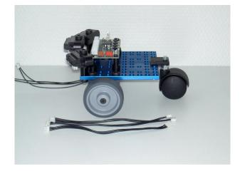
The sensors are connected to the connections An0 to An3; the motors are connected to the connections Mot0 and Mot1. In order that the supplied software will run without any changes being required, the connection configuration should be as follows:
